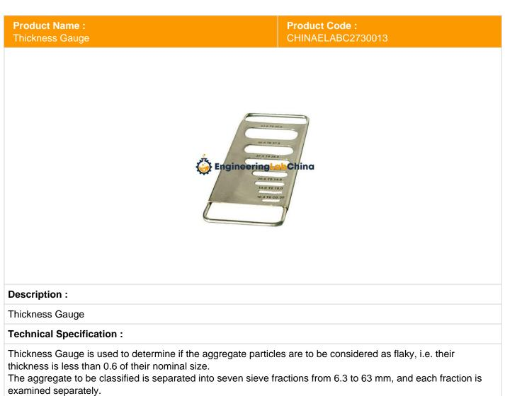
Slot sizes are 4.9 x 30 mm, 7.2 x 40 mm, 10.2 x 50 mm, 14.4 x 60 mm, 19.7 x 80 mm, 26.3 x 90 mm and 33.9 x 100 mm.
