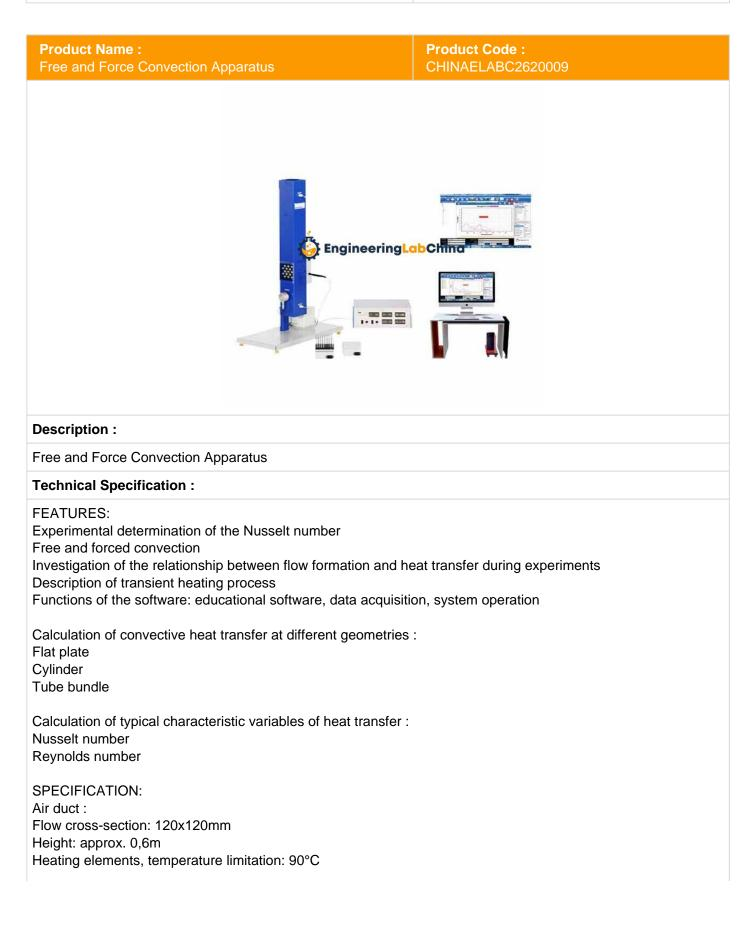
Tube bundle : Number of tubes: 23 One tube in variable position is heated Heating power: 20W Heat transfer area: 0,001m2
