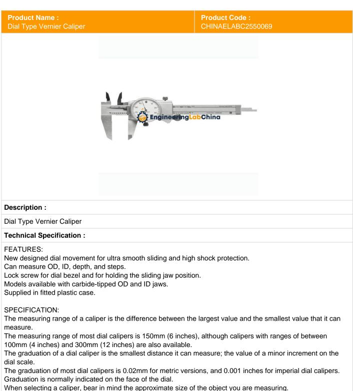
To measure larger objects, you will need a caliper with a larger measuring range.
