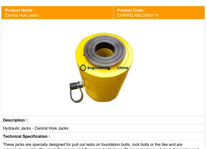
extensively used by Structural Engineers and Research Institutions. These jacks have a hole in the centre and are designed for dual operation. The hand pump is specially designed with two control lines i.e. one for extraction and the other for retraction. Separate control valves are provided. A calibrated load gauge is provided with each jack to read the load directly. Lifting handles are provided on jacks and pumps for ease of transportation.
