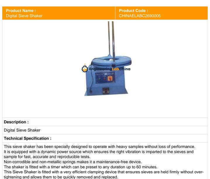
The vertical movement is fixed to ensure the sample spends maximum time on the sieve surface.
